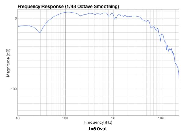
Based on 6" Supro, 6x9 oval (like in an automobile) speaker used in some early amplifiers (Supro).
