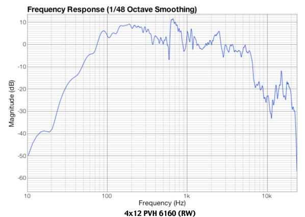
Based on: Older model Peavey 5150 4x12 cabinet loaded with four Sheffield 1200 speakers.
