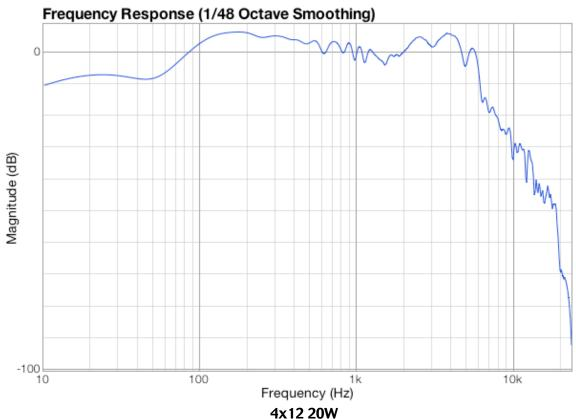
Based on: Marshall with 4x12 low-power 20 Watt Greenbacks.
