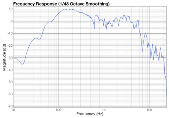
4x12 1960B T75 (RW) Based on: Straight Marshall 1960 loaded with four Celestion G12T-75s.
