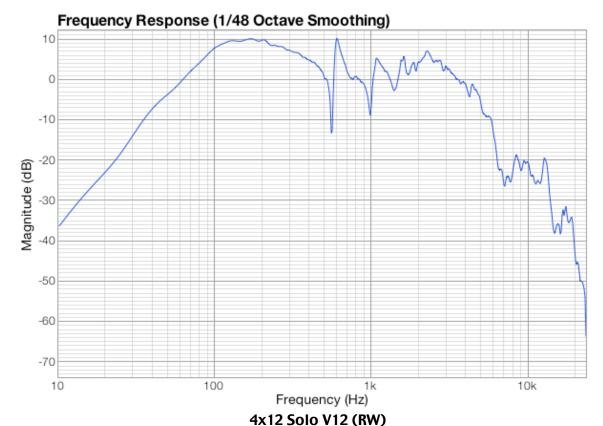
Based on: Soldano 412B loaded with four Eminence Legend V12s. A lot more high-end than the S12X version. It's a front-loaded cab with lots o' resonance so you may need to back the mics off a bit more than usual.
