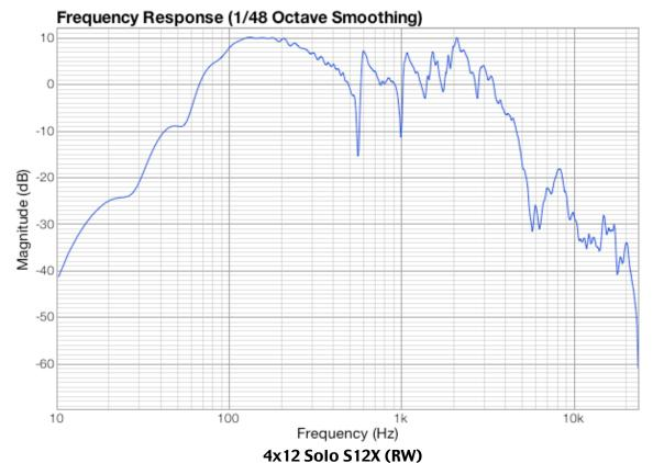
Based on: Soldano 412B loaded with four Eminence–made S12Xs. S12Xs were stock in the older cabs. Give this one a little more distance than you might normally, the cab resonance is pronounced up close and the speakers have a notch in the upper mids between 4–8KHz. Nice for taming fizzy guitars.
