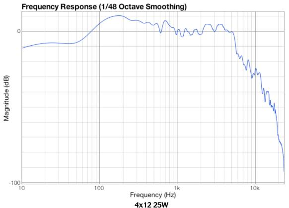
Based on: Marshall with 4x12 25 Watt Greenbacks, 1970's.
