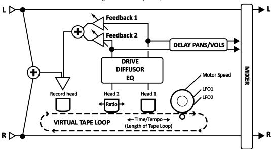
Figure 5-11 – The Tape Delay Block
