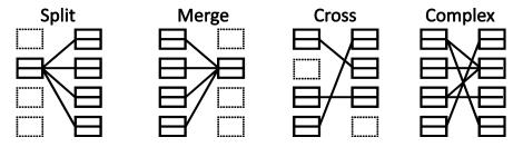
Figure 4-6 – Cables can CROSS one another without issue. Routings can be as COMPLEX as required.
