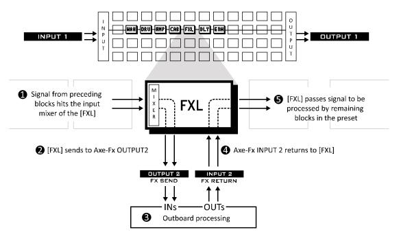
Figure 5-13 – Effects Loop Routing
