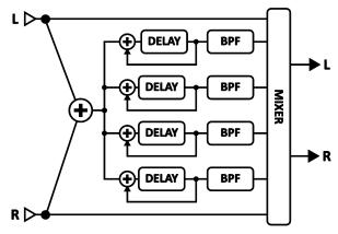
Figure 5-37 — The Resonator Block, Shown in its MONO INPUT MODE.
