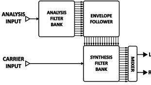
Figure 5-41 - The Vocoder Block
