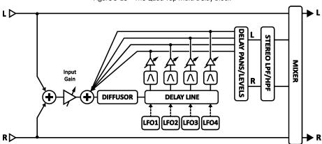
Figure 5-18 - The Quad Tap Multi Delay Block
