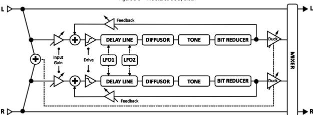
Figure 5-9 - The Stereo Delay Block
