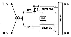
Figure 5-39 – The Rotary Speaker Block
