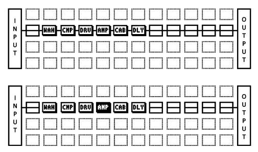
Figure 4-5 – Two otherwise identical presets shown WITH and WITHOUT connector cables between the blocks.
