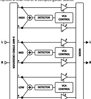
Figure 5-17 – Stylized view of the Multiband Compressor
