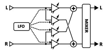
Figure 5-24 – The Pan/Tremolo Block
