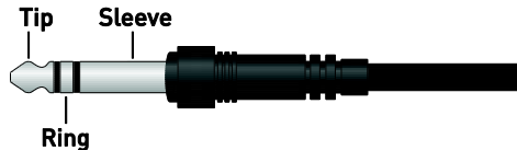
Figure 7-1: TRS Cable, AKA “Balanced” or “Stereo” Cable End. Regular guitar cables will NOT work for expression pedals!
